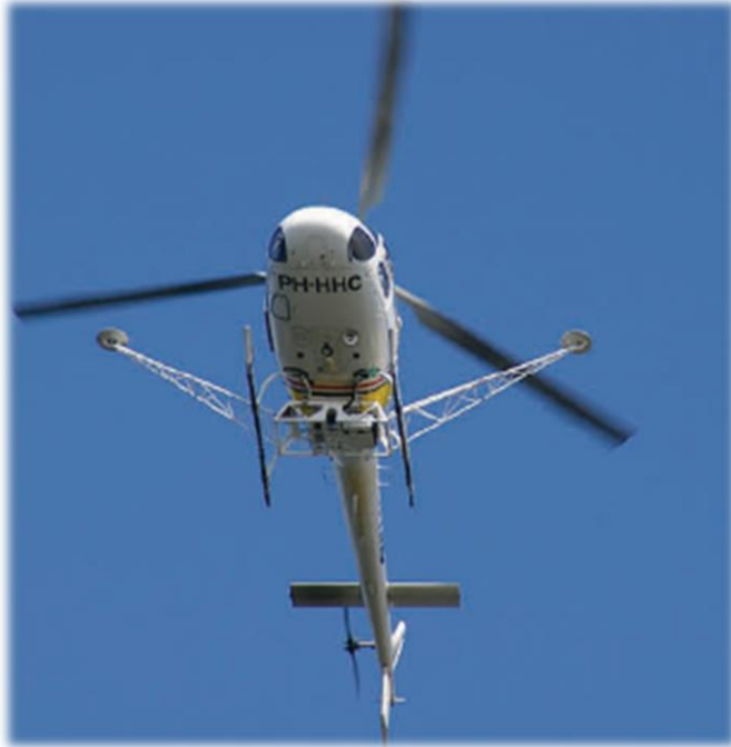
Aerial LiDAR Survey at 40 scans per metre
