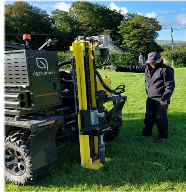
Soil Sampling to one metre deep
